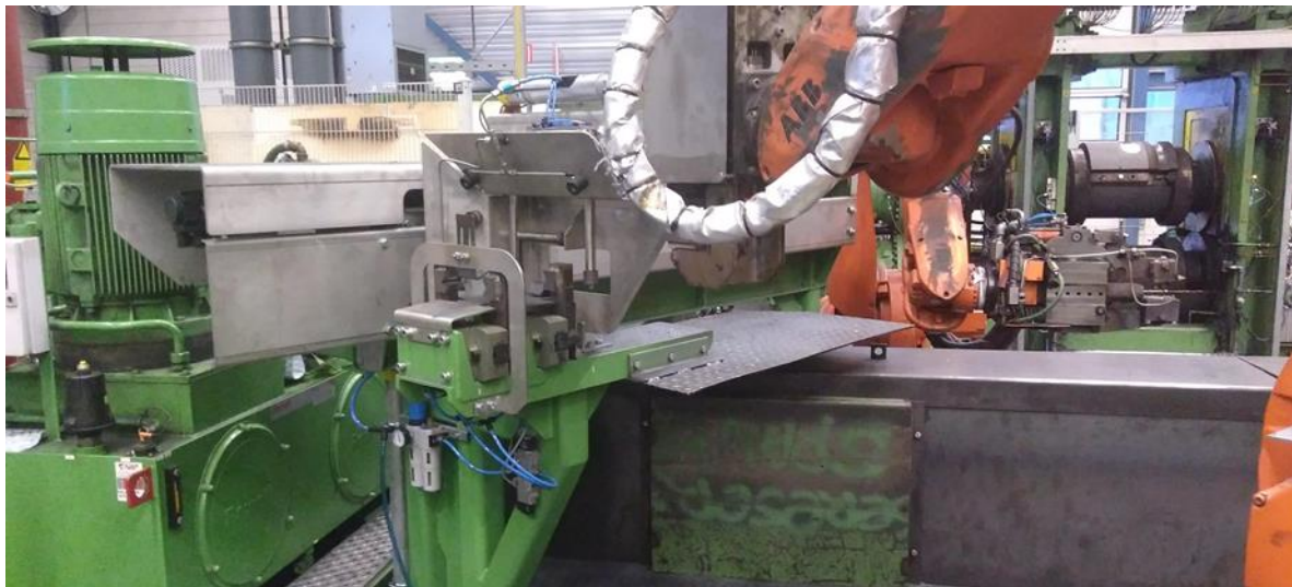
Figure 17. Measurement machine integrated into production line
