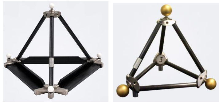
Figure 12. Artefact for contact and non-contact sensors.
